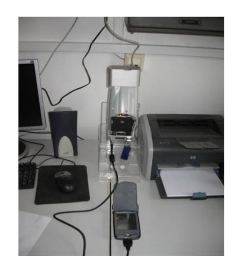
X-MET 3000 TXR+ portable XRF spectrometer: 40 kV tube Rh–anode; PIN Si diode detector, Peltier cooling; 270 eV resolution for  $K_{\alpha}$  line of Mn (5.89 keV); measurement spot size about 30 mm<sup>2</sup>; Hewlett-Packard (HP) iPAQ personal data assistant (PDA) for software management and data storage.
